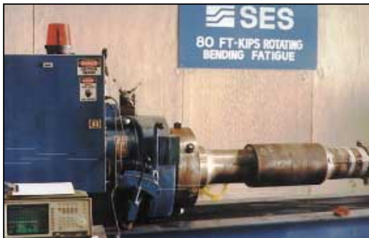
Fatigue Testing of Riser Connector
