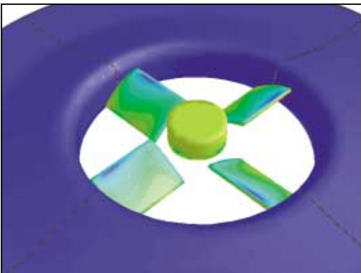
Figure 2. Fan model analysis results. Colors represent pressure distribution on the suction side of the blades.
