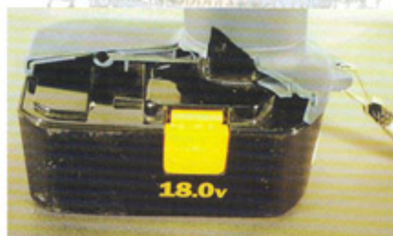
Fatal failure of a battery-operated drill when dropped on its handle
