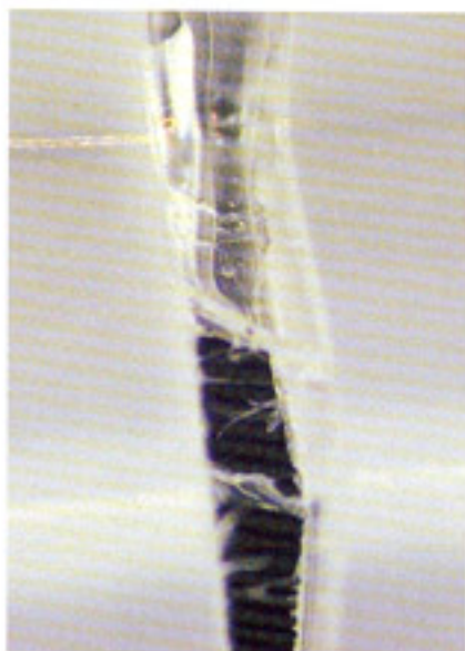
Crack morphology in a failed HDPE valve
