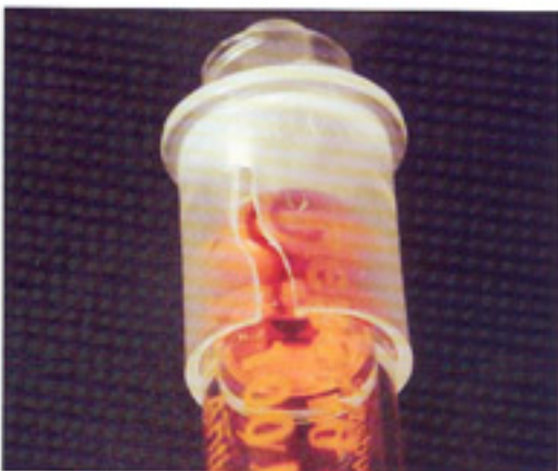
Time-dependent cracks in pharmaceutical syringe components
