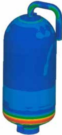
*Creep Analysis of a Vessel Using Finite Element Analysis*
