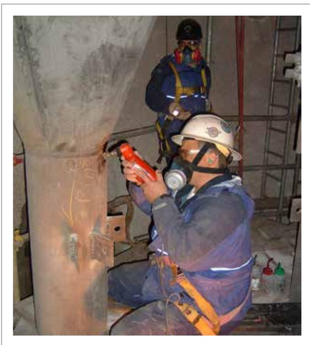
*Conducting on-site Field Metallurgical Replication*
