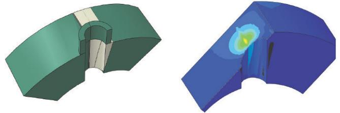
Model of header seamweld through tube ligaments showing an internal region of creep damage in weld HAZ
