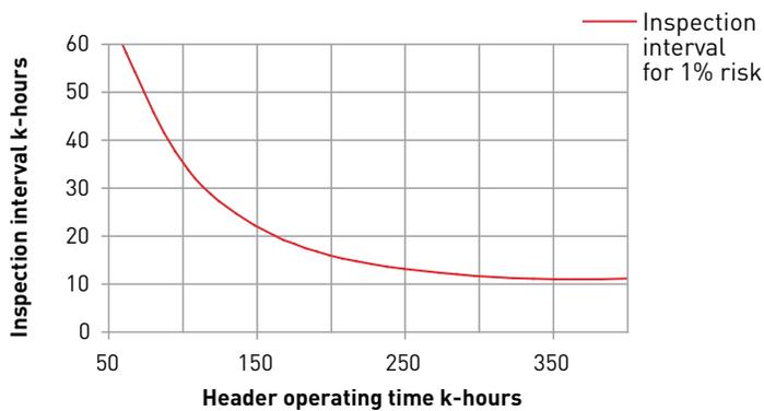
Calculated header inspection interval for uniform risk (material, stress, cycle and temperature dependent)
