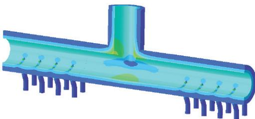
Stress analysis of header showing nozzle and tube penetration stress concentrations
