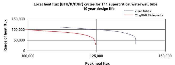
*Effect of heat flux cycles and internal fouling on waterwall tube life*
