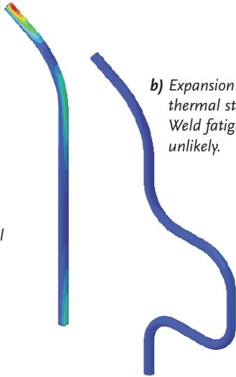
*b) Expansion loop reduces thermal stress by 80%. Weld fatigue highly unlikely.*
