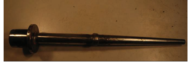
Fatigue failure of a thermowell due to vortex-induced vibration.
