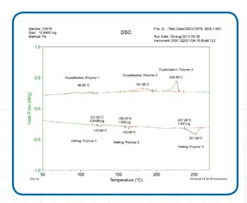
Standardized tests include oxidative induction time, blend compositional analysis, crystallization and melting temperature, glass transition temperature (Tg), the enthalpy of crystallization and melting, and non-isothermal crystallization and melting behaviors. The instrument can also be used to complete more research-oriented evaluations such as determination of thermal conductivity, isothermal crystallization behavior and the development of Avrami crystallization models.
