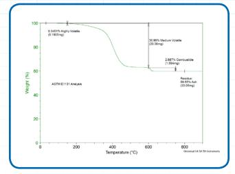
detect degradation induced during aging. This tool is used by SES, in combination with accelerated aging, to anticipate degradation mechanisms that can lead to premature failure.
