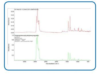
cure in adhesives, transesterification reactions in polyesters, and in some cases it is possible to identify oxidation and decomposition of the organic compounds in polymers. Perhaps the most common usage of the FTIR is for contamination analysis when working to uncover the root cause(s) of a failure.
