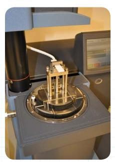
be measured with a DMA. Measuring material damping is particularly useful when evaluating the dynamic properties of elastomers. For composites, a DMA can be used to determine the degree to which a composite has been cured.
