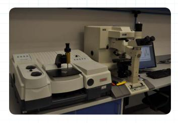
Fourier Transform, Infrared Spectroscopy (FTIR) is an analytical characterization technique that is used to identify unknown non-metallic materials. FTIR makes identification possible because each functional group (C-H, C-N, C-O, etc.) has a specific excitation band when exposed to infrared light. The FTIR technique is used to reconstruct a polymer material and to identify unknown compositions. Advanced sampling techniques can be used to determine degree of
