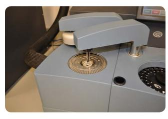
The DSC is an extremely versatile instrument which produces data for product/component design, failure analysis and material compatibility assessment.
