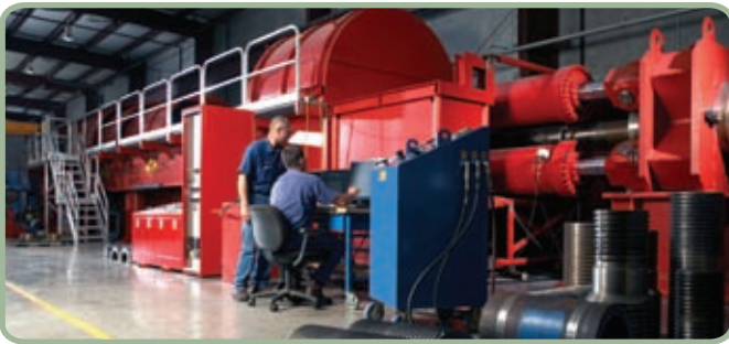
Six Million Pound Tension / Compression Test Frame
