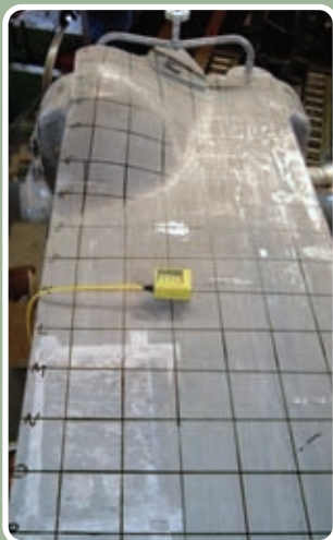
A 6-inch grid on the surface of a vessel explosion bulged aluminum plate fin heat exchanger. The grid was used to support a finite element analysis model.
