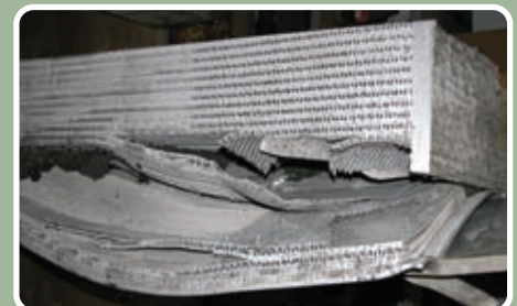
A cross section through the bulged region of an aluminum plate fin heat exchanger showing the separation at the low and high pressure passages.
