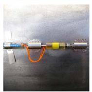
Vibrating wire strain gages are often used to monitor pipelines in remote environments and for measuring over extended periods of time.
