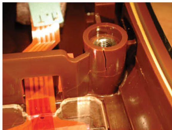
Figure 1: Cracked boss in device caused by sustained strains in PC.
