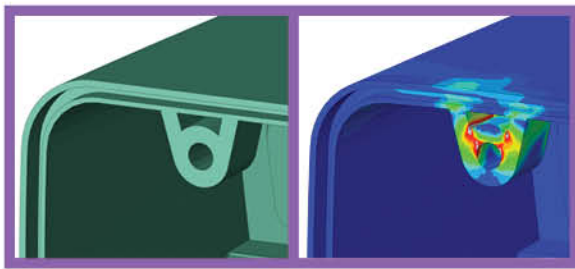
Figure 3: Finite element methods are often used to calculate sustained stress/strain in complex geometries.
