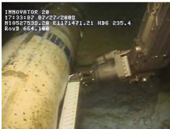
Dent profile being measured subsea
