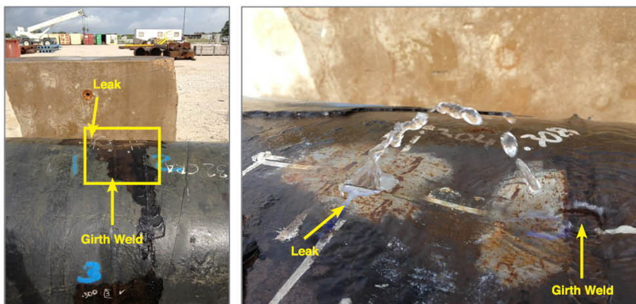
Leak failure in dented test sample after being subjected to cyclic pressures
