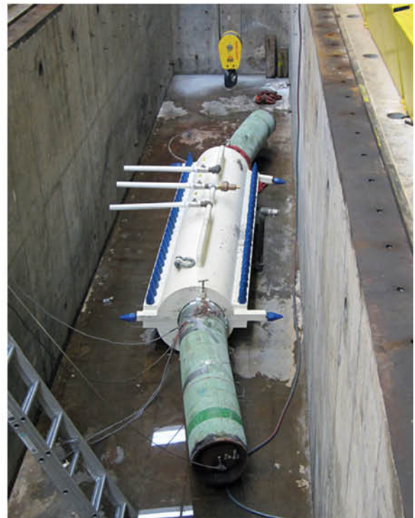
Sleeve-reinforced sample in test pit prior to burst
