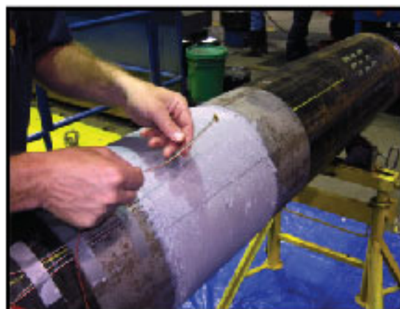
Figure 3: Machined corrosion with inter-layer strain gage installation
