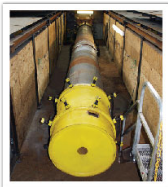
36" sample in a Resonant Bending Fatigue Machine
