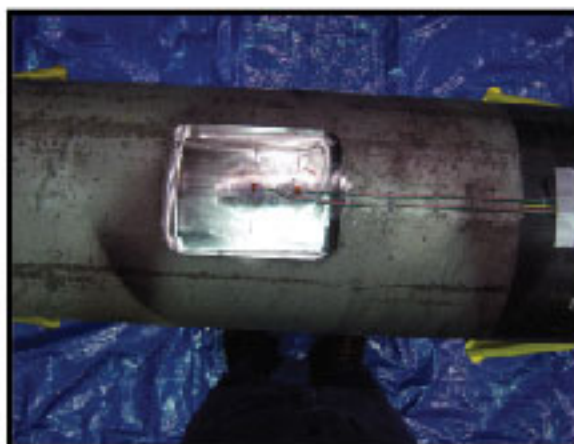
Figure 3: Machined corrosion with inter-layer strain gage installation
