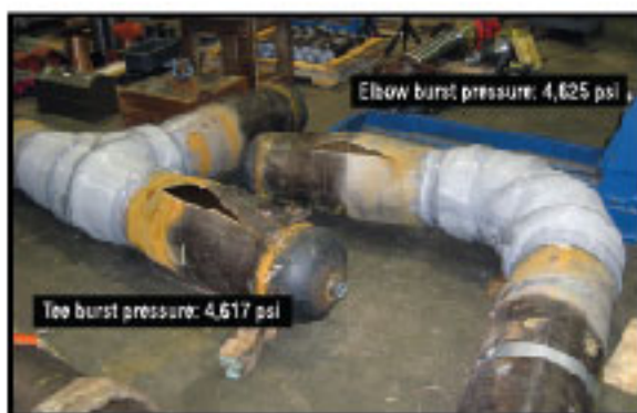
Figure 2: Reinforced pipe fitting tests
