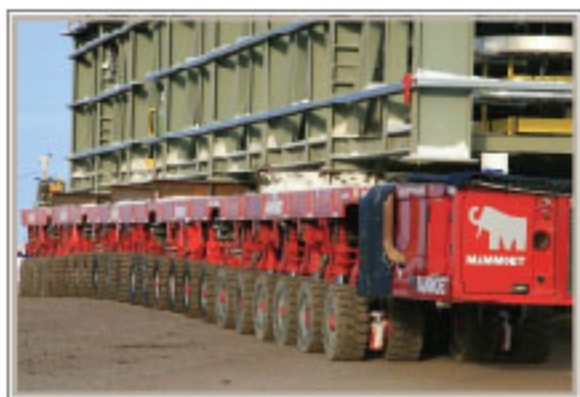
SPMT Configuration/Roof Structure In Transit
