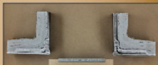
Reinforced in-plane Sample (after 4.7 inches displacement at 124.0 kip-feet bending)
