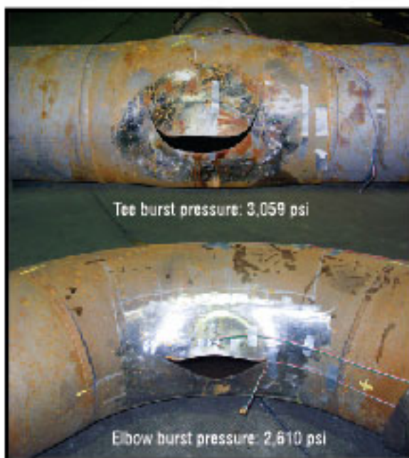
Figure 1: Unreinforced pipe fitting tests
