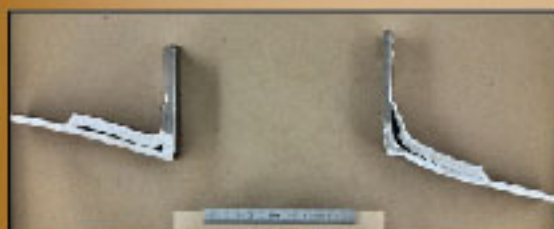
Unreinforced in-plane Sample (after 13.3 inches displacement at 88.6 kip-feet bending)
