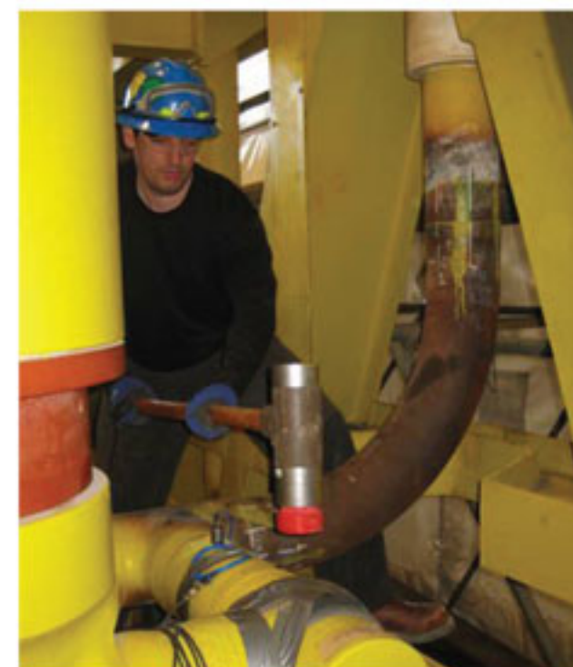
Figure 2: Impact testing of a large valve system using a modal sledge hammer.
