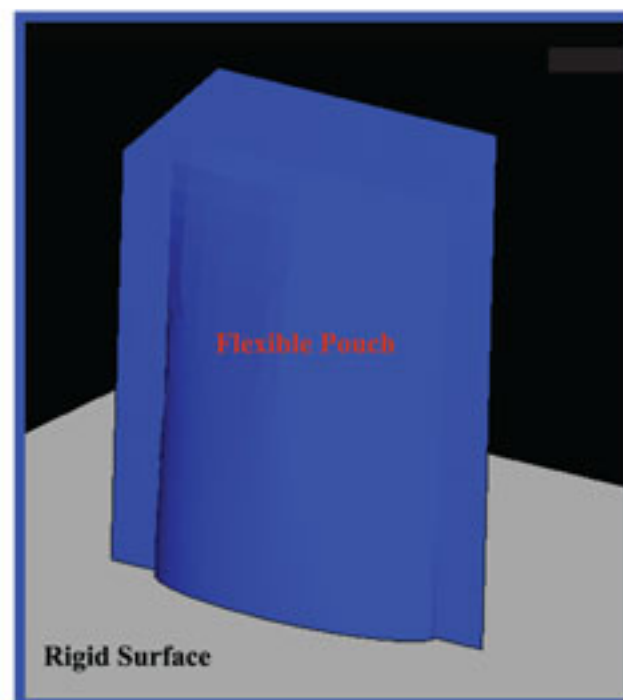
Figure 6: Finite element model of a fluid-filled flexible pouch
