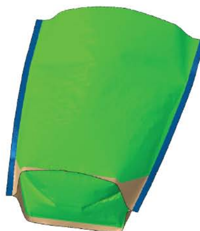
Figure 4: Simulation of pouch filled with liquid product prior to sealing and retort processing
