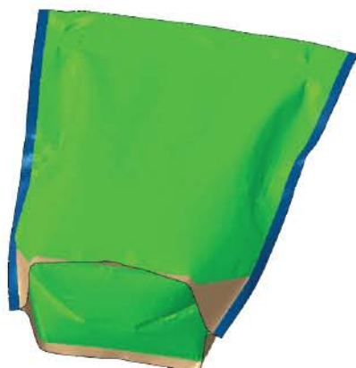
Figure 5: Simulation of final closure heat seal and deformed shape of pouch, prior to retort
