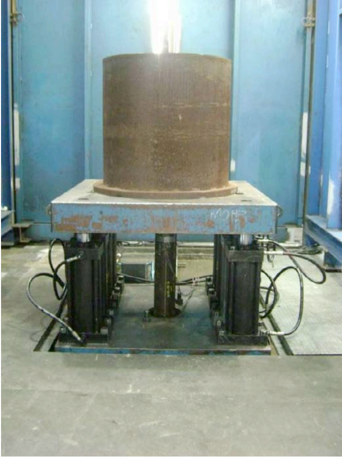
Fig. 5. Conventional slips installed in small load frame
