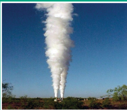
Dispersion of gas plume from a burst test is simulated to determine safe working zone
