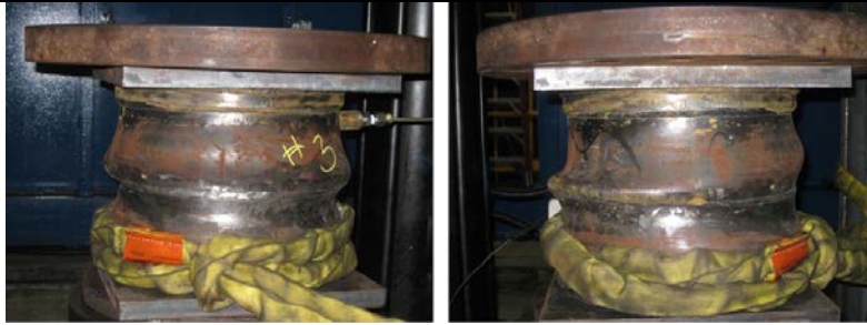
Figure 5. Sample 3 (girth weld in center) after sub-scale buckling test of 12-inch NPS pipe
