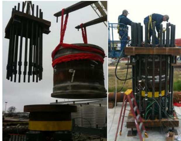
Figure 6. Assembly of load frame for full-scale testing
