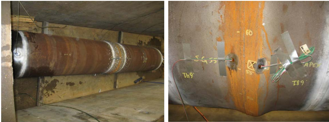
Figure 7. Sample to be pressure cycled in burst pit with pups, end caps and instrumentation.
