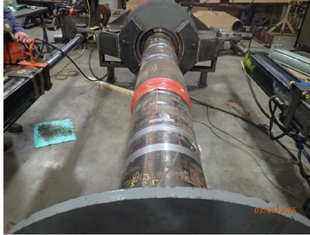
Figure 6. Sample in the reeling frame (installation moment loading)
