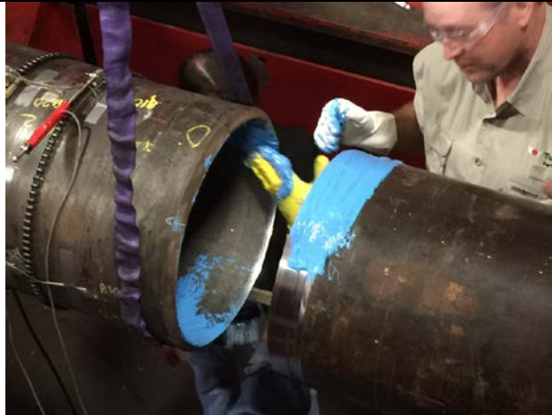
Figure 3. Application of lubricating epoxy on Sample 1 prior to joining (406-mm OD x 21.4-mm Wall Thickness, Grade X52 (Actual Yield Strength of 71.5 ksi)).
