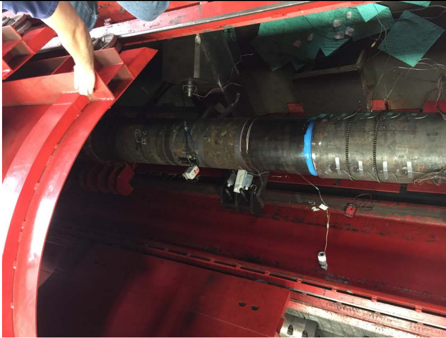
Figure 8. Interference Connection Sample LP1 Prior to Testing
