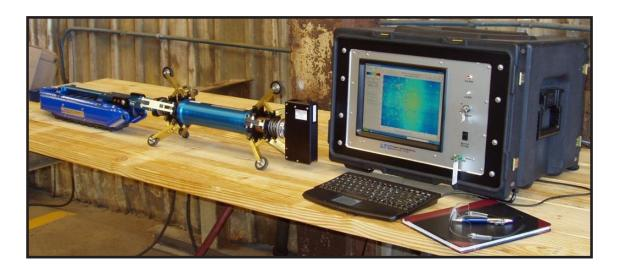
Utilizing the high-performance Bore Erosion Measurement and Inspection System (BEMIS™) tool, developed by Laser Techniques Company LLC, we are capable of rapidly, accurately, and quantitatively mapping the internal surface of 2" - 22" diameter pipes. The BEMIS™ laser sensor is the only system on the market that accurately measures and maps the ID of pipe/tubing, rotating at high speed through the length of a tubular, typically generating upwards of 5000+ data points per revolution.
