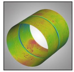
The result is a high-resolution 3D map of the component inner surface and a rapidly delivered report summarizing the anomalies and their location on the tube, providing a digital record of the asset.
