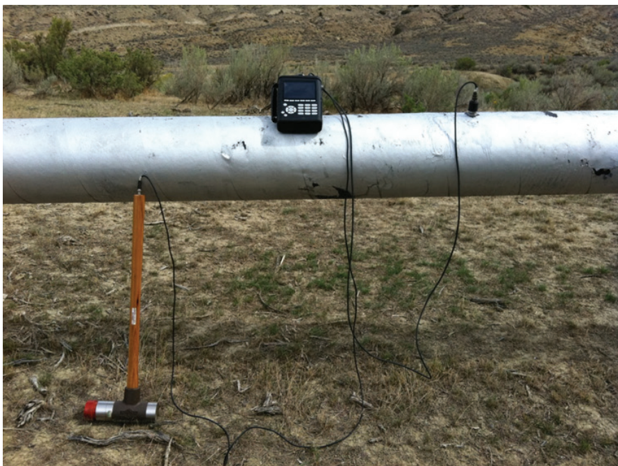
Figure 7: Test equipment mounted on a pipe span for field measurement of the damping factor
