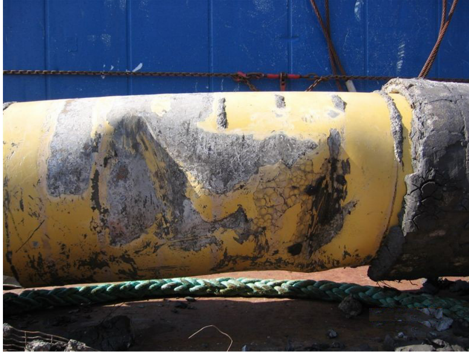
Figure 9 – Photograph of damaged 30-inch gas pipeline off coast of Israel [16]
