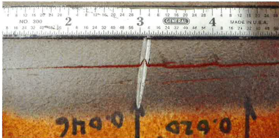
Figure 3: Photograph of Feature 8988 from Sample 3 showing MPI indication after second grinding pass. Numbered scale divisions are inches.
