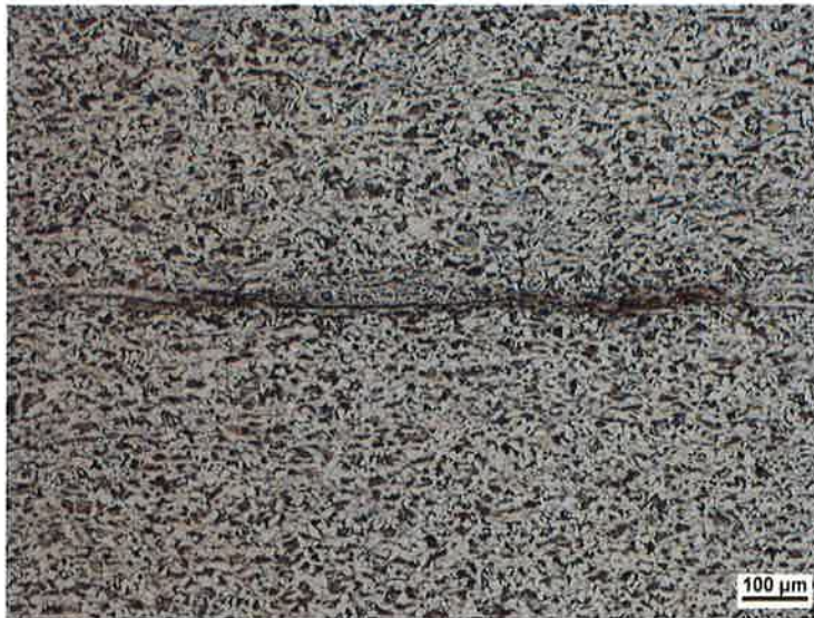
Figure 5: Photomicrograph of flaw from Sample 1 (Feature 2644). Etchant is 2% Nital; original magnification is 100x.
