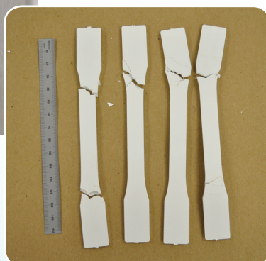
ABS test specimens cracked by exposure to a quaternary disinfectant
