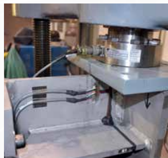
Once designed, each pedestal sensor was then calibrated in a load frame in our laboratory.
