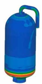
Creep Analysis of a Vessel Using Finite Element Analysis
