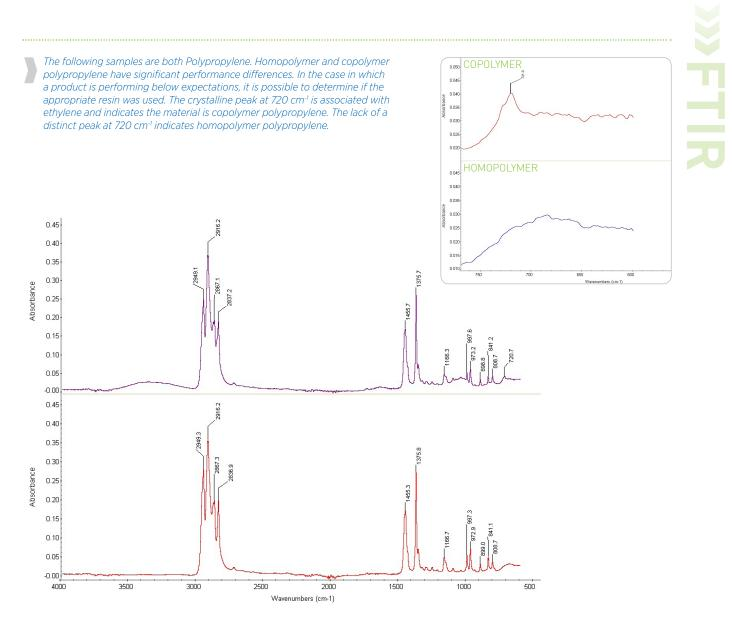
SES conducts analysis using both standardized and customized methodology. A list containing common test methods is shown below. Employing a database with 1000s of library spectra, SES is capable of identifying most unknown materials.
