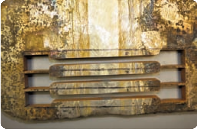
Figure 3B Creep Specimens cut out of material extracted from process equipment
