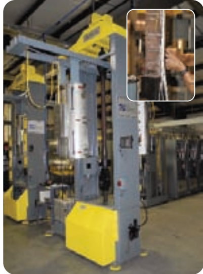
Figure 2 100 kip creep test specimen with thermocouples and AE sensor mounted
