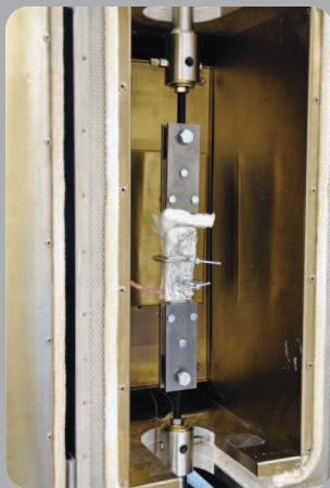
Figure 7 Local heating of composite specimens during tensile testing.
