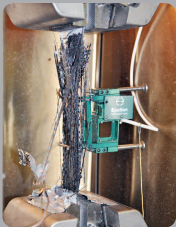
Figure 7 Local heating of composite specimens during tensile testing.
