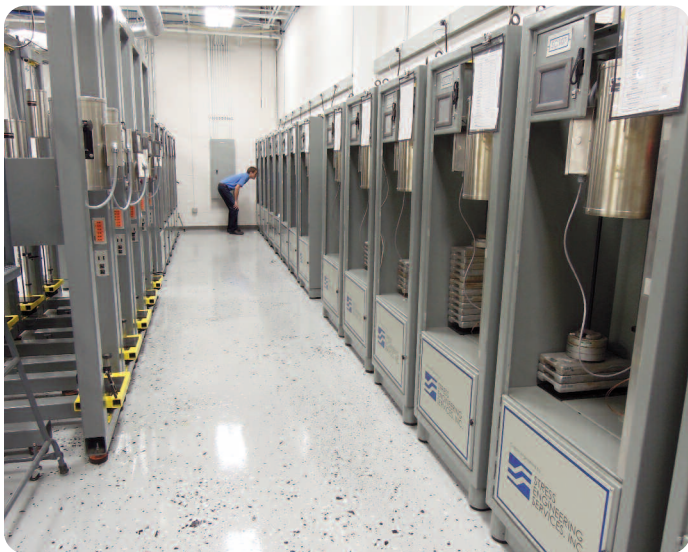
Figure 5 Stress Engineering Services creep testing laboratory.
