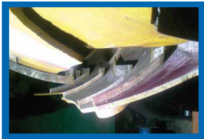
Figure 3: Brittle Fracture during pressure testing
