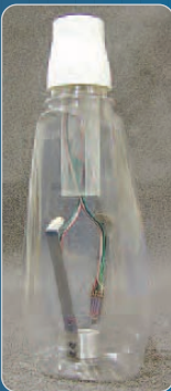
Miniature data acquisition system for measuring bottle labeling force
