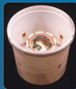
MicroDAQ installations used to measure force, temperature, acceleration and battery usage
