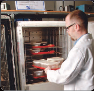
Accelerated aging chamber
