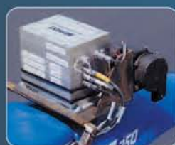
MicroDAQ installations used to measure force, temperature, acceleration and battery usage
