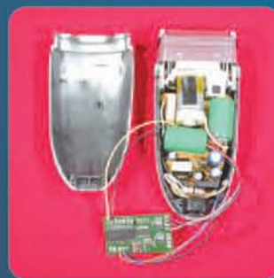
MicroDAQ installations used to measure force, temperature, acceleration and battery usage
